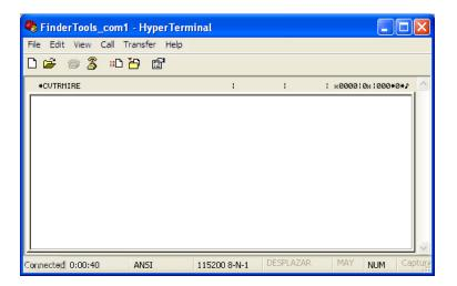
3. Keep pressing the ESC key in the keyboard when turning on the field meter, and the following picture will be shown on the PC, then you can stop pressing the ESC key.
