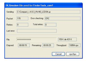
6. As the updating has finished the following picture will appear. Then the field strength meter has to be rebooted and the RS232 cable has to be disconnected from the PC and field meter.
