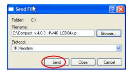
5. Press SEND button after you select the file. Then press the DOWN key on keyboard of the field meter and the updating will start.
