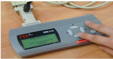
7.- Finally, push on the "Program" button. The transfer of the new software will begin. It finishes resetting the module PRO20X. The new software is ready to be used.
